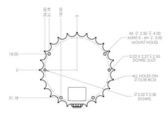
The sensor has 4 x M3 mounting holes and 2 x 2.0 mm dowel pin holes
