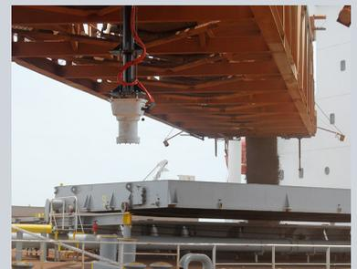
The weather in Pilbara is very dry and hot, and video technologies and Lidar sensors are adversely affected by dust. Navtech's sensors operate flawlessly in all environments and require minimum maintenance.
