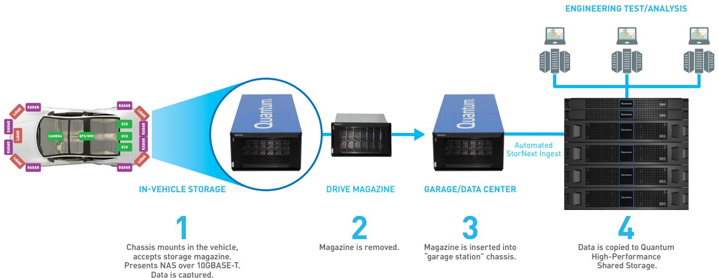
The removable drive magazine simply and quickly uploads car data to the development team from the storage chassis mounted in the garage station.
