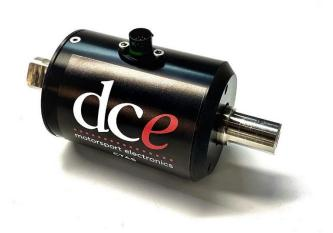
The DC Electronics CTAS device is designed to be fitted in line with the steering column and can be used to transmit torque and steering angle signals to the vehicle datalogger to aid with vehicle set up, or it can be used to directly connect these signals to the DC Electronics range of power steering ECUs, when used as part of an electric power steering system.
