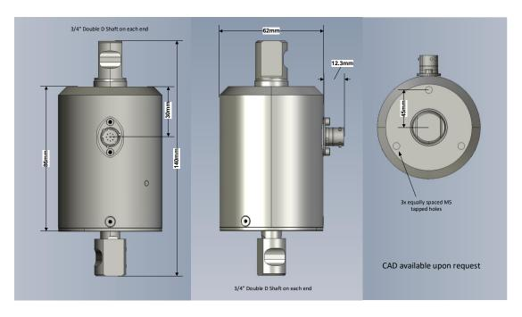
To stop the sensor rotating, the CTAS body should be mounted to the chassis with the 3 x M5 tapped holes. These holes should be at the opposite end of the sensor to the steering wheel.
